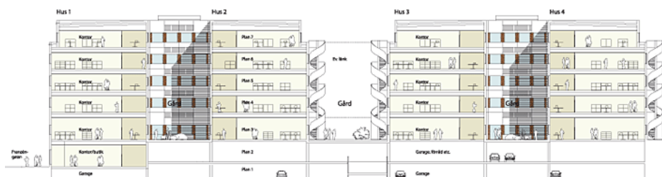
Figure 1. A drawing showing the Västerport project with its seven-storey buildings.
